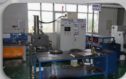
Laser Welding 激光焊接
